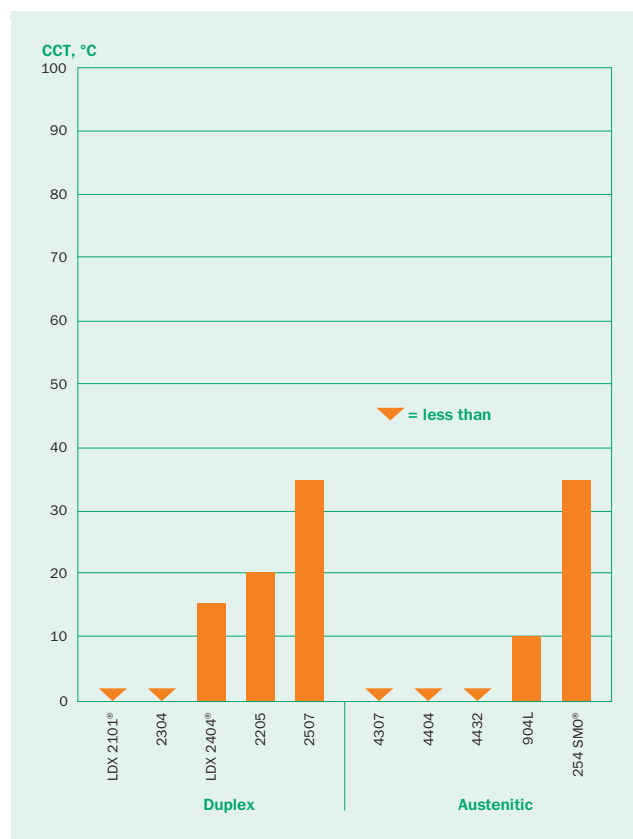
Fig. 6. Typical critical crevice corrosion temperature (CCT) according to ASTM G 48 Method F. Test surfaces dry ground to 120 mesh. CCT varies with product form and surface finish.
