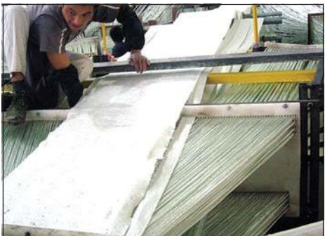
Glassfibre rovings and matting reinforcement
