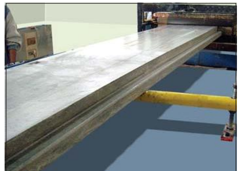
Final pultruded resin glassfibre Dura Slab
