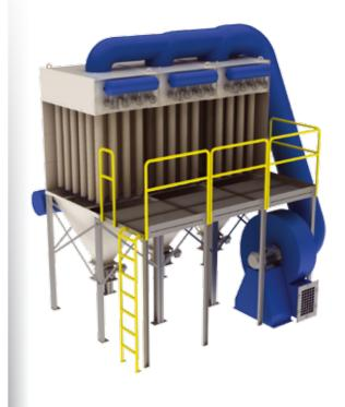
Dust collector M2000-3-54 is a three box-shaped device. It is used for central filtration in various industrial areas with non-stop operation. It is equipped with the standalone fan and dust hoppers with support construction.
