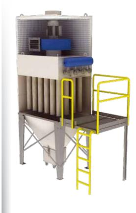
Dust collector M1500-1-18 is a one box-shaped device. It is used for local or central filtration in various industrial areas with non-stop operation. It is equipped with the built-in fan and dust hopper with support construction.
