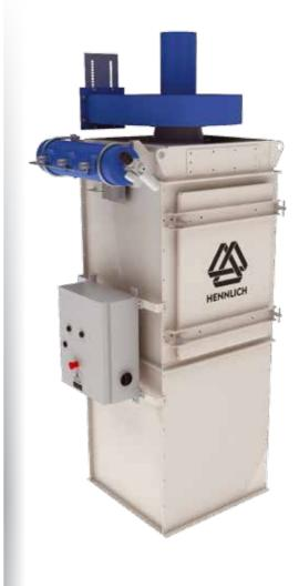
Dust collector P1500/5,5 is a box-shaped device. It is used for local filtration - dedusting of storage silos, belt conveyor transfer points, welding operations etc.
