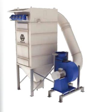
Dust collector M2000-1-24 is a one box-shaped device. It is used for local or central filtration in various industrial areas with non-stop operation. It is equipped with the standalone 37 kW fan, hopper with support construction and dust collection box.
