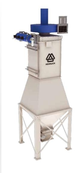
Dust collector P1500/KR3 is a box-shaped device. It is used for local filtration - dedusting of storage silos, belt conveyor transfer points, welding operations etc. It is equipped with the support construction, dust hopper and rotary feeder.
