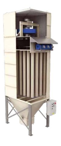
Dust collector M1500-1-18 is a one box-shaped device. It is used for local or central filtration in various industrial areas with non-stop operation. It is equipped with the built-in fan and dust hopper with support construction.
