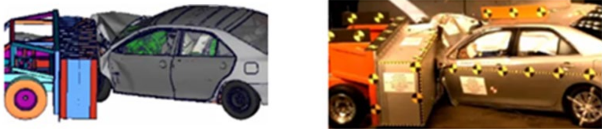
Figure 1 - Frontal Oblique Test Configuration
