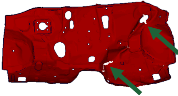
Figure 17 – Right Oblique – Local Material Failure for CM-Composite 1
