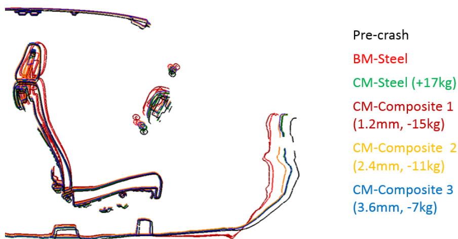
Figure 13 – Left Oblique Intrusion- Baseline vs. CM-Steel and CM-Composite
