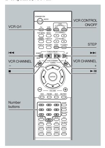
After pressing **VCR CONTROL ON** on the remote control, you can perform the following operations on the VCR.
