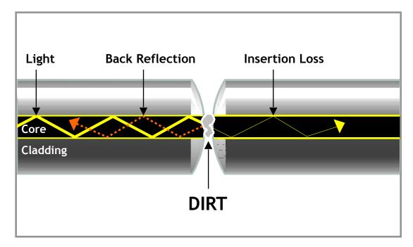
A single particle mated into the core of a fiber can cause significant back reflection and insertion loss
