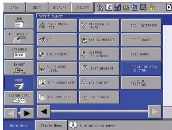
Figure 1-12 OPERATION AREA MONITOR select
