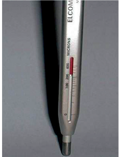
Figure 17: Magnetic system „Pull off Gauge 157“ Elcometer Instruments Ltd. Manchester
