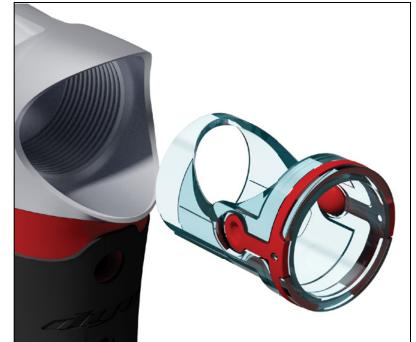
remove the eye pipe/detent system from the front of the M2 and unclip the detents for a thorough cleaning. Reinstall the detents, and eye pipe after you have sufficiently cleaned the detents and breech.
