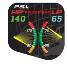
The screen will read "Processing" and display HP and LP psi. When done, press the center of the joystick, and continue to scroll through the Data Settings menu.
