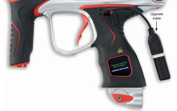
You can customize the boot screen on your M2 with any photo you like. The full color provides remarkable detail and image resolution. Before you can download a photo onto the board it will first need to be converted to a .bmp file sized 128 x 128 pixels. You can use any number of free online programs such as the one listed below to convert your photo. http:// image.online-convert.com/convert-to-bmp
