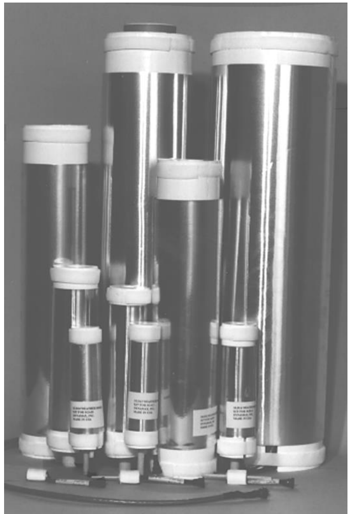
Figure 1.1 - Dynagages: Range of sizes
