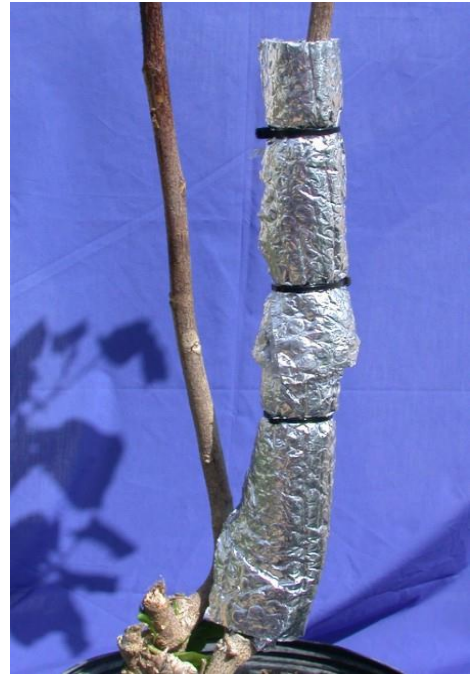
Figure 4.7 - Bubble foil Shield installation over sensor
