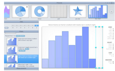
Figure 3.9: Victor's Drawing Dynamic Visualizations. The left panel shows a recording of the actions taken by the designer. Designers can create dynamic visualizations through a combination of modifying the steps in the recorded actions, and direct manipulation of the graphics in the center panel.
