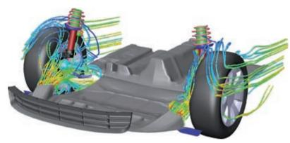
Figure 3: Simulation of the air flow to the brakes
