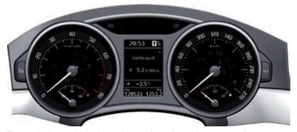
Figure 10: Indication of the used gear is shown in the cluster instrument as well as optimum time for gear change according to consumption
