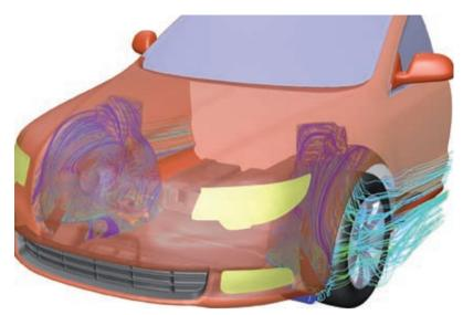
**Figure 2:** The air flow towards the brakes was simulated early on in the development phase and subsequently validated to achieve an optimum cooling of the brake calipers and thus the optimum braking performance
