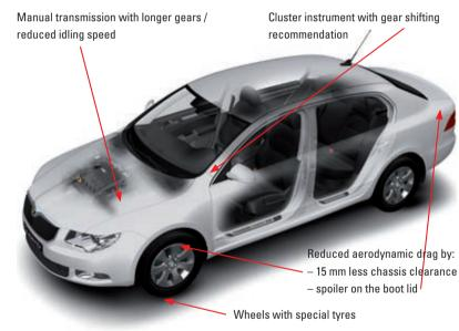
Figure 9: In the Greenline version the Superb has 0,6 I less fuel consumption per 100 km
