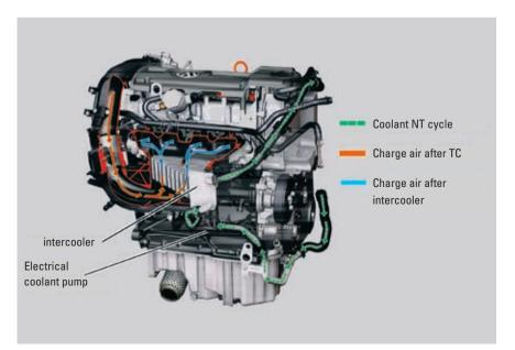
Figure 4: 1.4-I-TSI: Low-temperature coolant circuit at back of engine and air flow in charge air cooler
