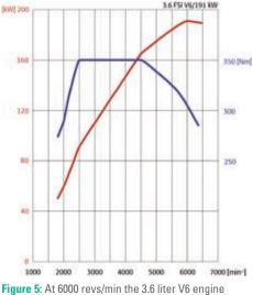
has a maximum power of 191 kW. The torque of 350 Nm is available from 2500 revs/min up to 4500 revs/min
