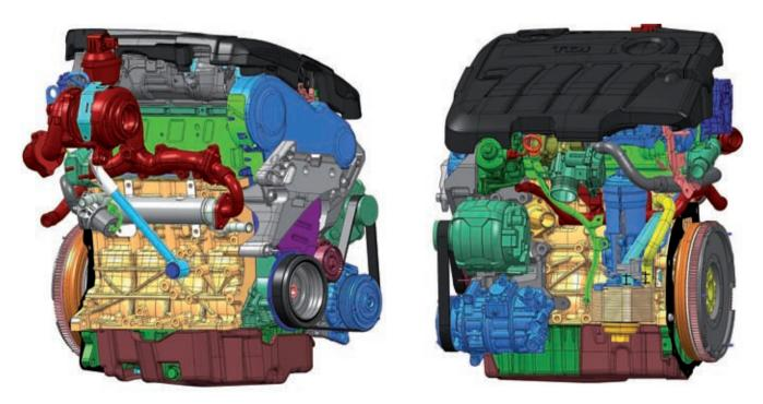
Figure 8: The new 2.0 liter/125 kW TDI with common rail technology, diesel particulate filter and compensation shaft module is the top Diesel engine
