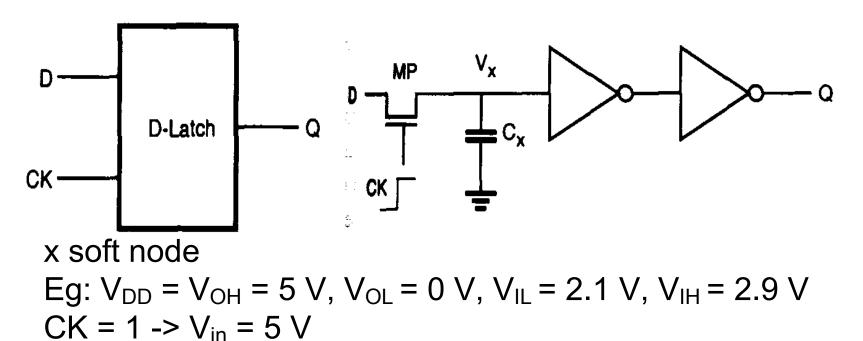
$C_x$  charge up  $V_x = 4.2$  V (poor conductor) ->  $V_{out} = 0$  V (1<sup>st</sup> inverter)  $V_{out} = 5$  V (2<sup>nd</sup> inverter)
