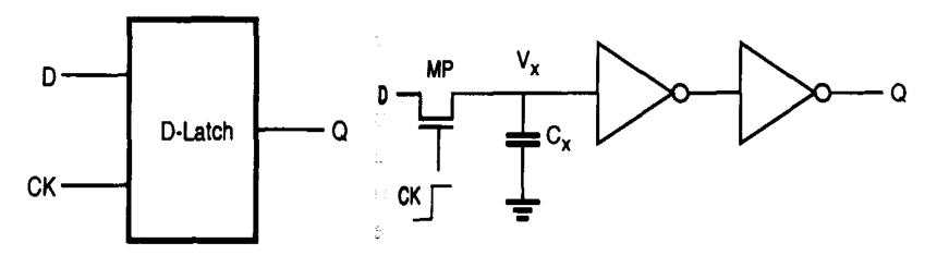
transistor turns off, logic high is preserved by  $C_x$ V<sub>x</sub> drops from 4.2 V -> to whatever (charge leakage) V<sub>Q</sub> = 5 V requires V<sub>x</sub> > 2.9 V C<sub>x</sub> must be restored
