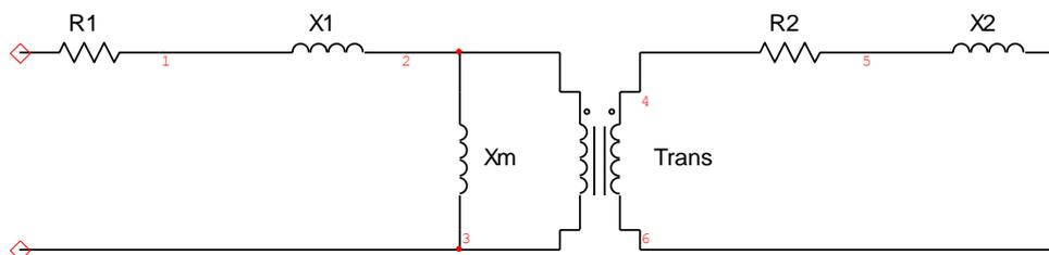
FIGURE 5 EQUIVALENT CIRCUIT OF WOUND ROTOR INDUCTION MAHCINE
