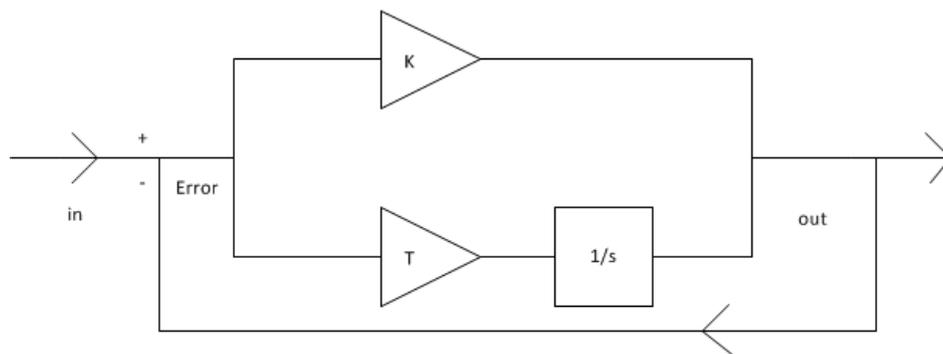
FIGURE 16 SCHEMATIC DIAGRAM OF A PI CONTROLLER (WIKI, 2014)
