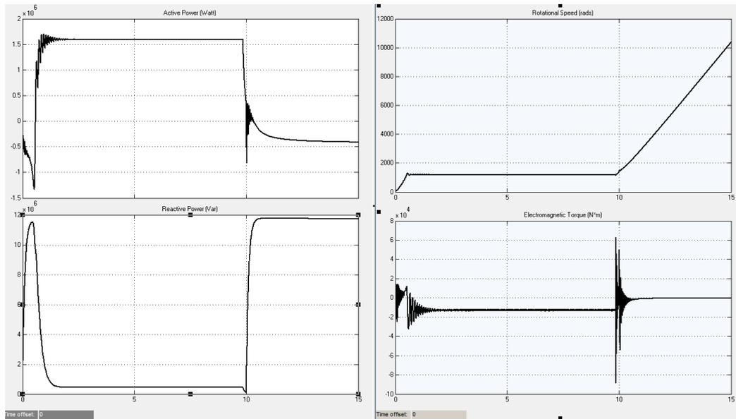
FIGURE 21 THREE PHASE FAULT TIME LENGTH: 0.15 SECONDS
