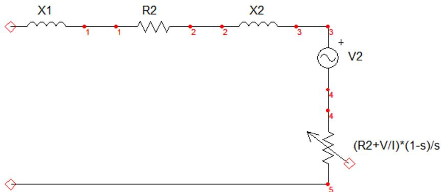
FIGURE 12 WOUND ROTOR INDUCTION MACHINE
