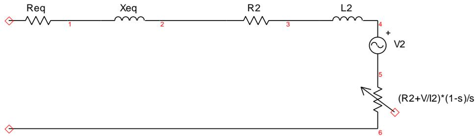
FIGURE 11 WOUND ROTOR INDUCTION MACHINE WITH VARIABLE SOURCE
