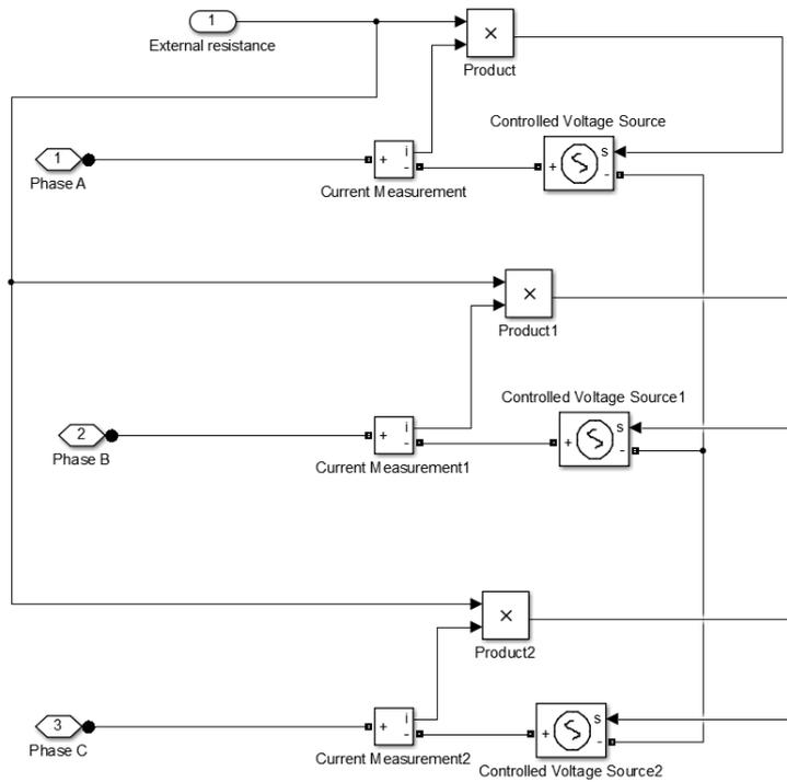
FIGURE 22 MODEL FOR EXTERNAL RESISTANCE
