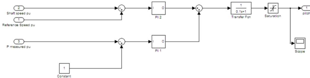
FIGURE 30 ACTIVE PITCH CONTROL SYSTEM
