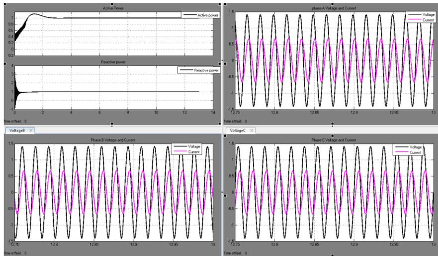
FIGURE 34 THREE PHASE VOLTAGE AND CURRENT WAVEFORMS IN ABC REFERENCE FRAME
