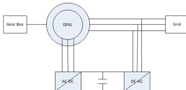
FIGURE 10 SCHEMATIC DIAGRAM OF DFIG
