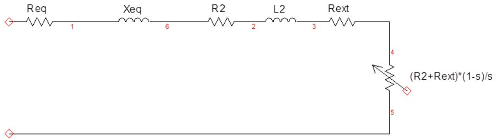
FIGURE 8 WOUND ROTOR INDUCTION MACHINE WITH EXTERNAL RESISTANCE
