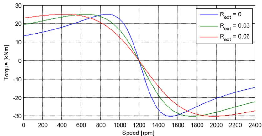
FIGURE 9 TORQUE AND SPEED CURVE OF VARIABLE RESISTANCE INDUCTION MACHINE (MOHIT, 2011)
