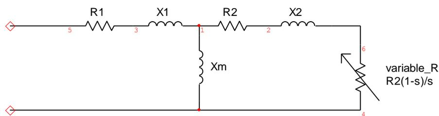
FIGURE 6 STATOR SIDE EQUIVALENT CIRCUIT OF WOUND ROTOR INDUCTION GENERATOR
