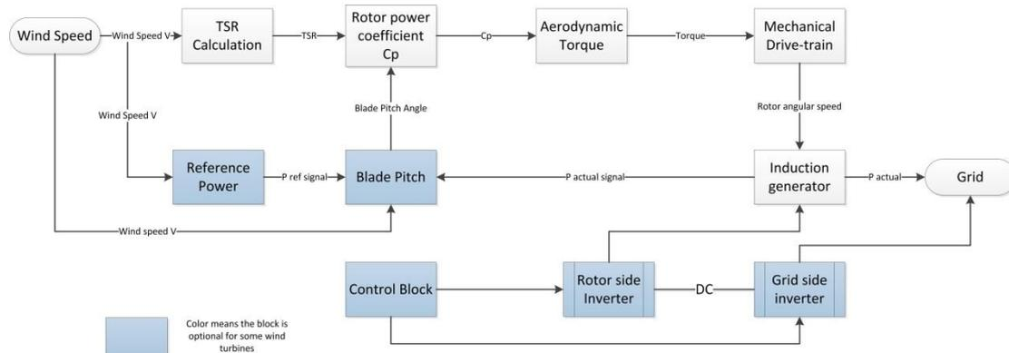
FIGURE 1 GENERIC STRUCTURE OF WIND TURBINE
