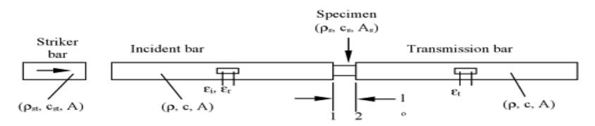
Figure 10.1. A schematic illustration of the Hopkinson bar set-up
