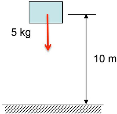
A falling body undergoes constant acceleration due to the force of gravity. Hence constant acceleration equations of motion apply.
