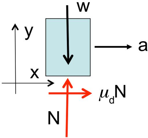
The weight is accelerated to the right by a friction force due to the sliding of the weight relative to the conveyor until velocities are equal.
