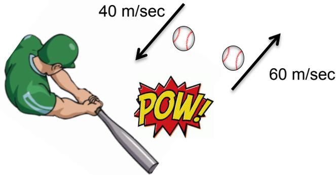
Assume inbound and outbound line of action is colinear and apply impulse momentum principle.
