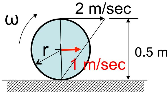
The kinematics of rolling contact that relates the linear velocity of the center of disk to its angular velocity is used to solve this problem
