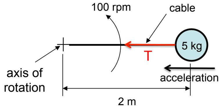
An object traveling in a circular path at a constant velocity is subject to an acceleration directed toward its center of rotation. This requires a radial force on the object.
