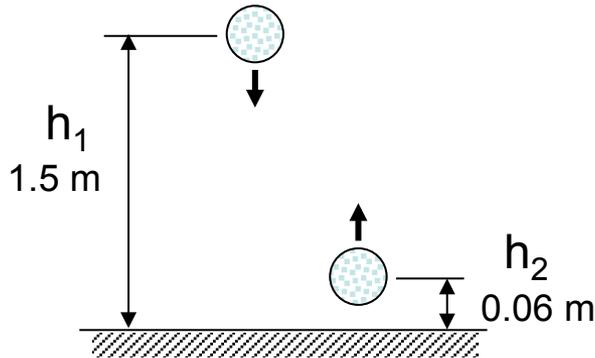
The coefficient of restitution "e" is a measure of the energy dissipated when a body impacts a surface and then rebounds.
