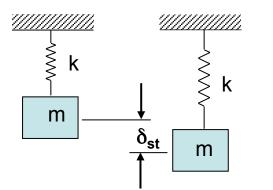
Period is one over the frequency. Calculate frequency for single degree mass on weightless spring.
