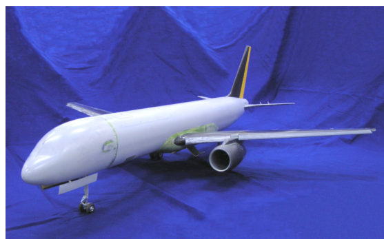
Figure 20. Photo of Generic Transport Model sub-scale flying testbed.
