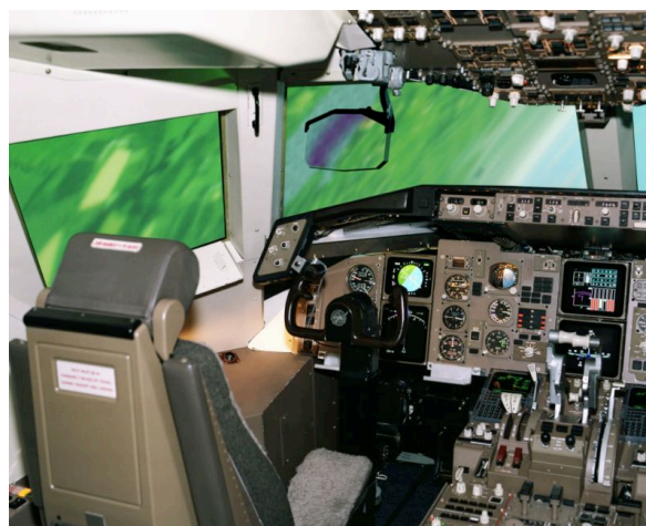
Figure 17. Photo of NASA LaRC IFD simulation cockpit.
