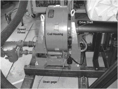
Figure 4 The SAJ eddy current dynamometer used for engine testing.
