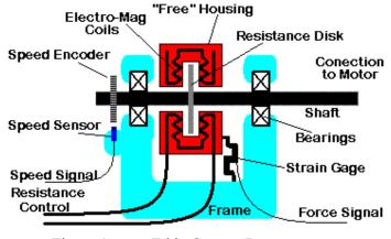
Figure 1. Eddy Current Dynamometer
