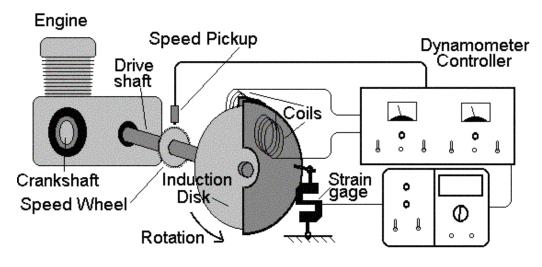
Figure 3 Schematic of a motorcycle engine and eddy current dynamometer
