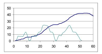
This is a plot of vehicle speed (dark thick line) in km/h versus time in sec, and Engine torque (in Nm) versus time for a test drive cycle. Notice that the engine operates at some torque loads more than others.
