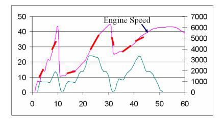
This is a plot of the engine speed superimposed on the previous torque curve. The red highlites indicate common speeds for some common torques: 7 Nm at 1800 rpm, 14 Nm at 4750 rpm, 24 Nm at 5000 rpm
