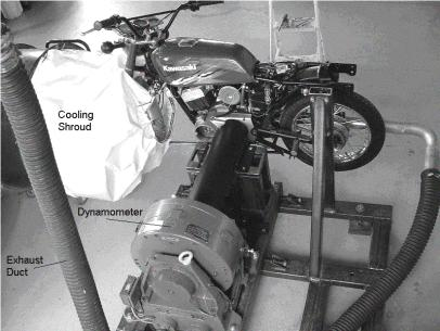
Figure 5 A Kawasaki HD-III mounted to the SAJ dynamometer.
