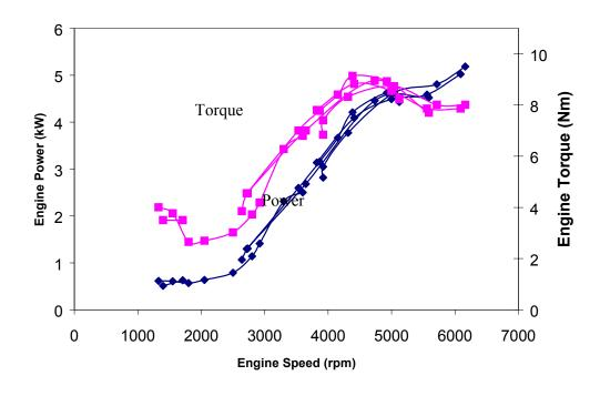
Figure 6 Power and Torque as a function of engine speed, WOT.
