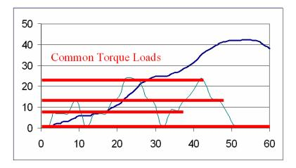
Common Torque loads (highlited in red) on this drive cycle are: 0 Nm (idle, or coasting), 7 Nm, 14 Nm, and 22 Nm. NOTE: We have neglected rolling friction and wind friction in the model
