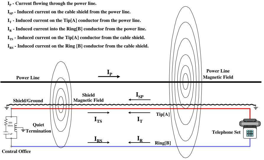
Note: 1. If the pair is well balanced, the opposing currents  $I_T$  vs  $I_R$  and  $I_{TS}$  vs  $I_{RS}$  will be equal and therefore cancel out.
