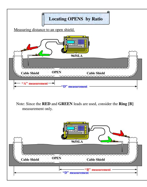
Requirement: Length of cable section under test must be known.
