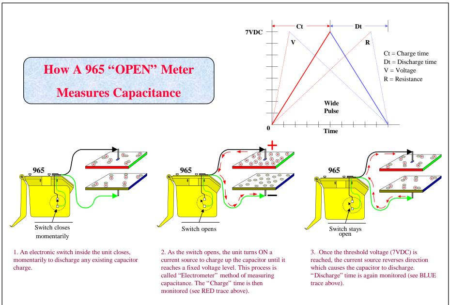
Note: Capacitance is directly proportional to the TIME it takes to charge and discharge the capacitor.
