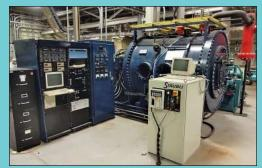
MSE Built Astro Furnace Spray Casting System
