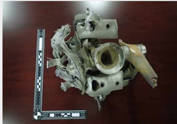
Figures 5 & 6 DLE 111 engine from the UAV used in the Marib attack, October 2016.
