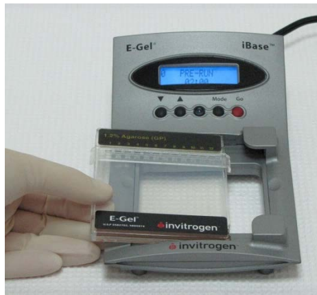
Slide cassette into electrodes
