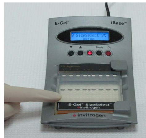
Press left side to secure
