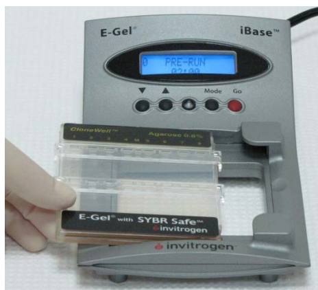
Slide cassette into electrodes
