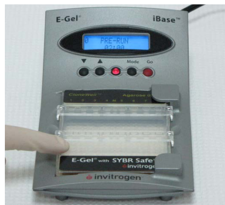
Press left side to secure
