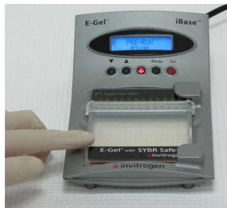
Press left side to secure
