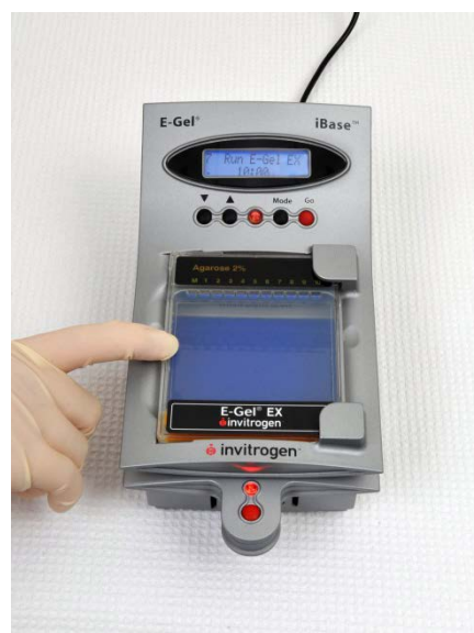
Press left side to secure
