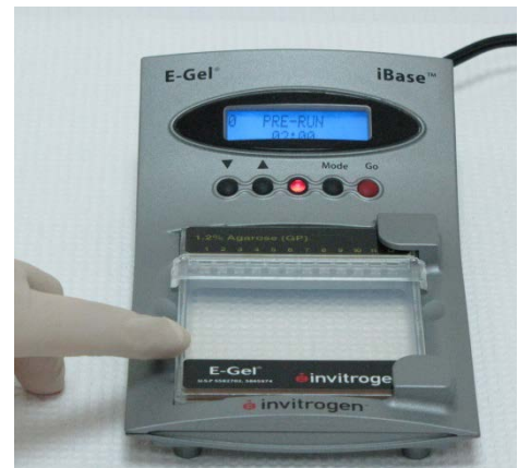
Press left side to secure
