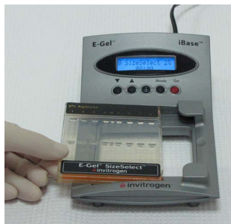
Slide cassette into electrodes
