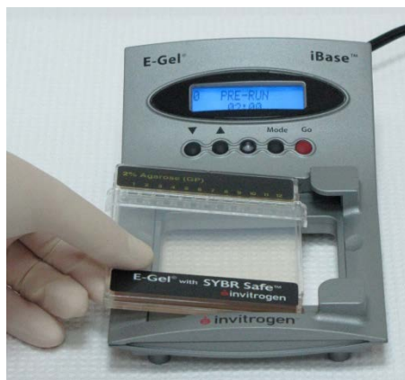
Slide cassette into electrodes
