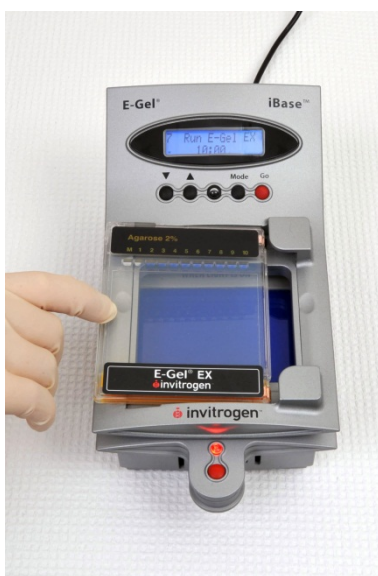
Slide cassette into electrodes
