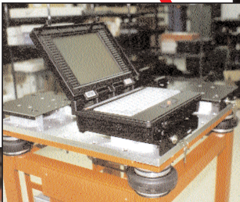
• SCR-350 on Test Table testing computer parts
