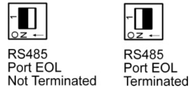
Figure 8: RS-485 EOL Switches
