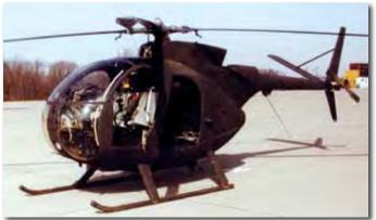
The OH-6 Cayuse was the primary A Company aircraft of the 1/245th from 1982 until 1986. The Cayuse was modified into the AH-6C attack and the MH-6B lift models. Under the SOA configurations, they were known as "Little Birds."
