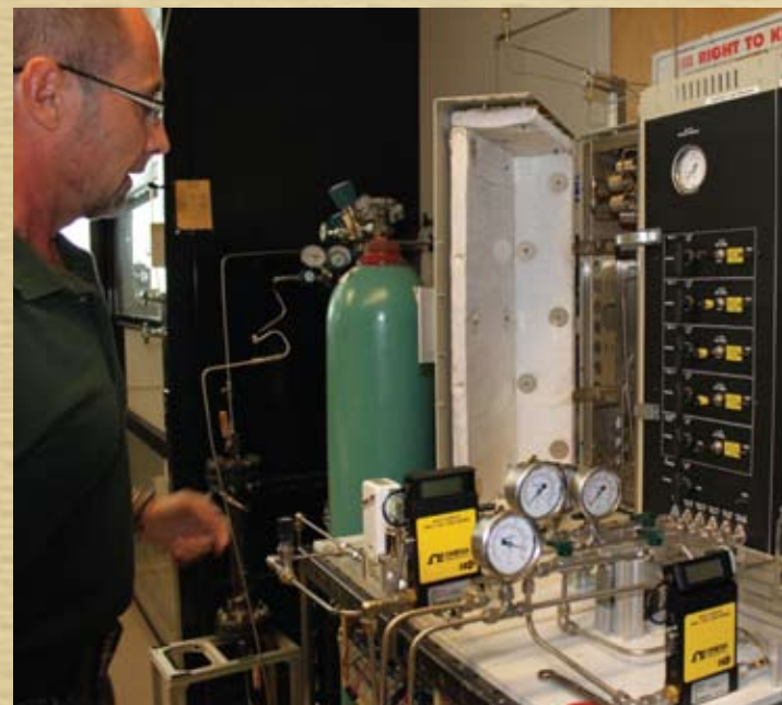
Professor John Wolan (examines) by the Fischer Tropsch bench-scale reactor and control system.
