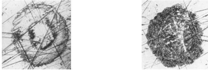
FIGURE 15.2 Effect of increased amplitude of fretting on fretting damage [6].
