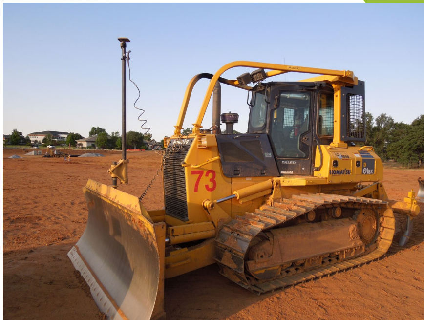
The Topcon 3D-MC 2 system provides readings roughly five times as fast as conventional machine-control systems and yields about three times the grading smoothness of other systems.
