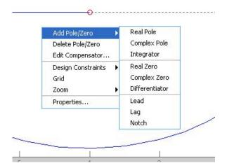
Right click and add a a real pole, and drag it to s = -5. Note the effect the added pole has. The Root Locus has been pushed closer to the Right Half Plane, and thus closer to instability. This shows that integral control hurts our transient perfor-
