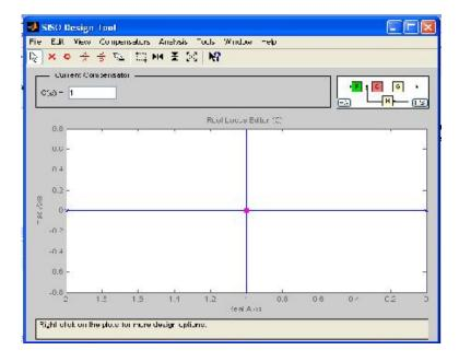
4 Take a moment and acquaint yourself with the layout of the GUI. The plot of the Root Locus has crosses at the location of the plant open loop (OL) poles (at s=0 and s=2), and squares at the location of the closed loop (CL) system poles for the current compensator, C(s).
