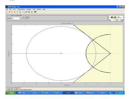
Now we have a compensator that can meet specs, provided we set the gain properly. Drag one of the CL poles (the squares on the Root Locus), and pull it until you are in the white region. Observe the compensator gain change as you move the CL poles; at the point you enter the region where both specs are met, the gain should be 4 (provided you're using the same plant and compensator from above).
