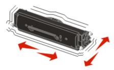
6 Install the new toner cartridge by aligning the white rollers on the toner cartridge with the white arrows on the tracks of the photoconductor and pushing the toner cartridge in as far as it will go. The toner cartridge *clicks* into place when correctly installed.
