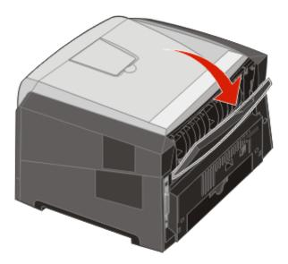
4 Press the two detents on the front right side of the machine, and swing the side door back.
