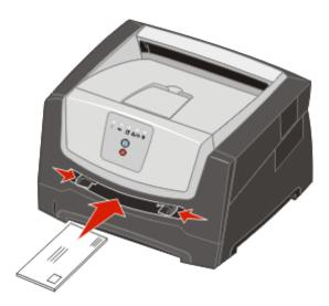
**10** Hold both sides of the print media close to the manual feeder, and push it into the printer until it automatically engages.
