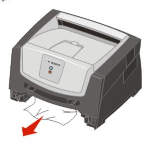
4 With the tray removed, press down on the green duplex flap to remove the jammed pages from the duplex area.
