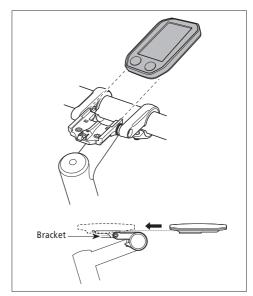
To remove the cycle computer, push the lever of the bracket firmly while sliding out the cycle computer.
