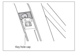
**2.** Insert the key into the key cylinder in the battery mount.
