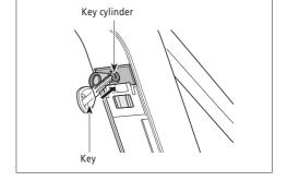
**3.** The battery detaches automatically when the key is turned clockwise and pushed in.
