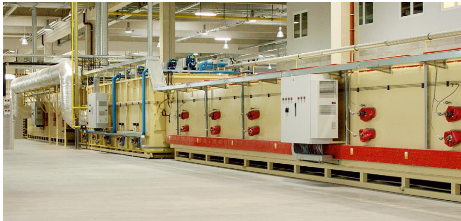
Continuously operating CAB furnace with five preheat and seven braze zones (Source: Seco-Warwick)
