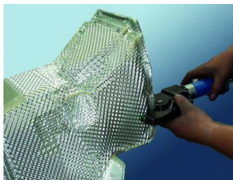
Joining of an aluminium heat shield with a hand held clinching tool
