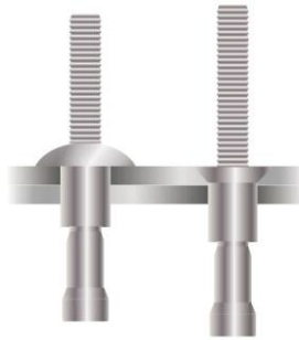
Self-plugging friction lock blind rivet: Protruding head (left) and countersunk head (right)
