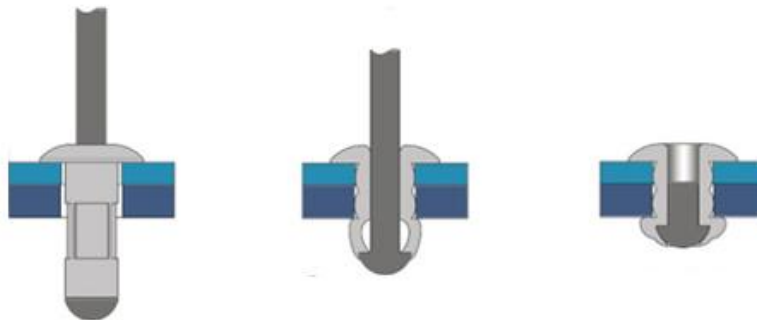
Standard blind rivets of the multi-grip design accommodate variations in material thicknesses
