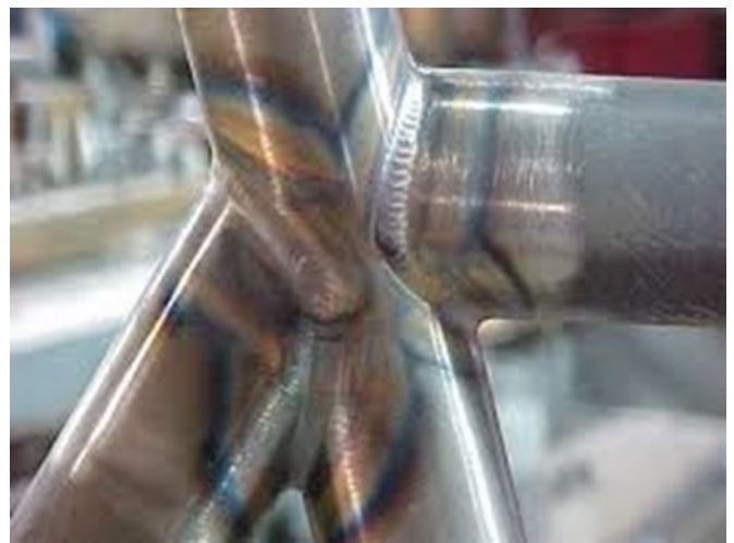
Excellent TIG welding on a fuselage joint cluster
