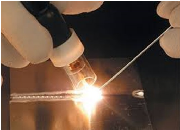
Filler rod is added to the argon protected weld puddle
