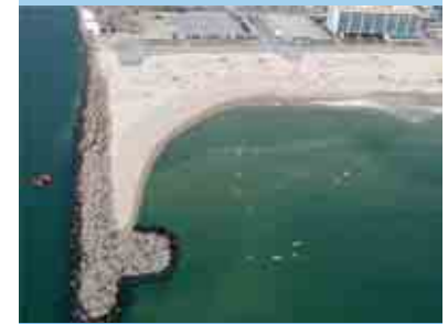
Conceptual photo showing the effect of the proposed spur on Rudee Inlet's north jetty
