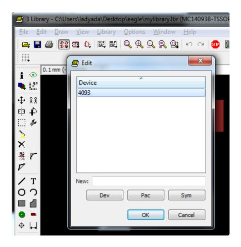
Once its open, click on New in the bottom right to create a new package variant. Select the new TSSOP14 we made
