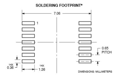
Looks like what we want are pads that are 0.36 by 1.26 and have 0.65mm pitch. So the pitch is right. Lets also check the spacing of the pads. Annoyingly enough, the diagram does not indicate the middle-to-middle spacing. We'll have to do a bit of math...
