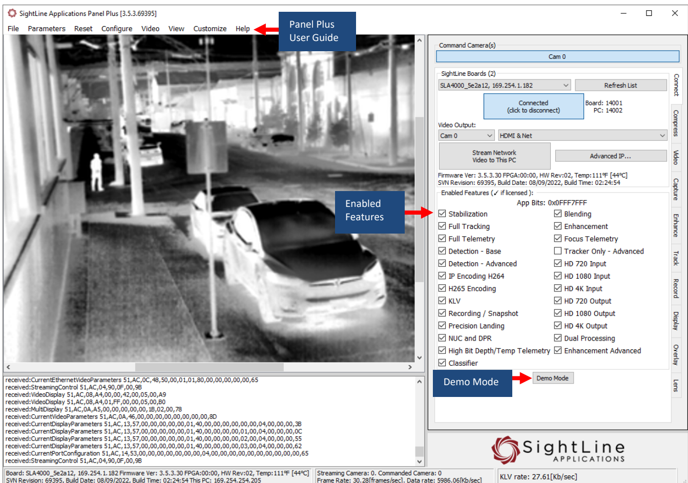
Figure 11: Panel Plus Connection to Board
