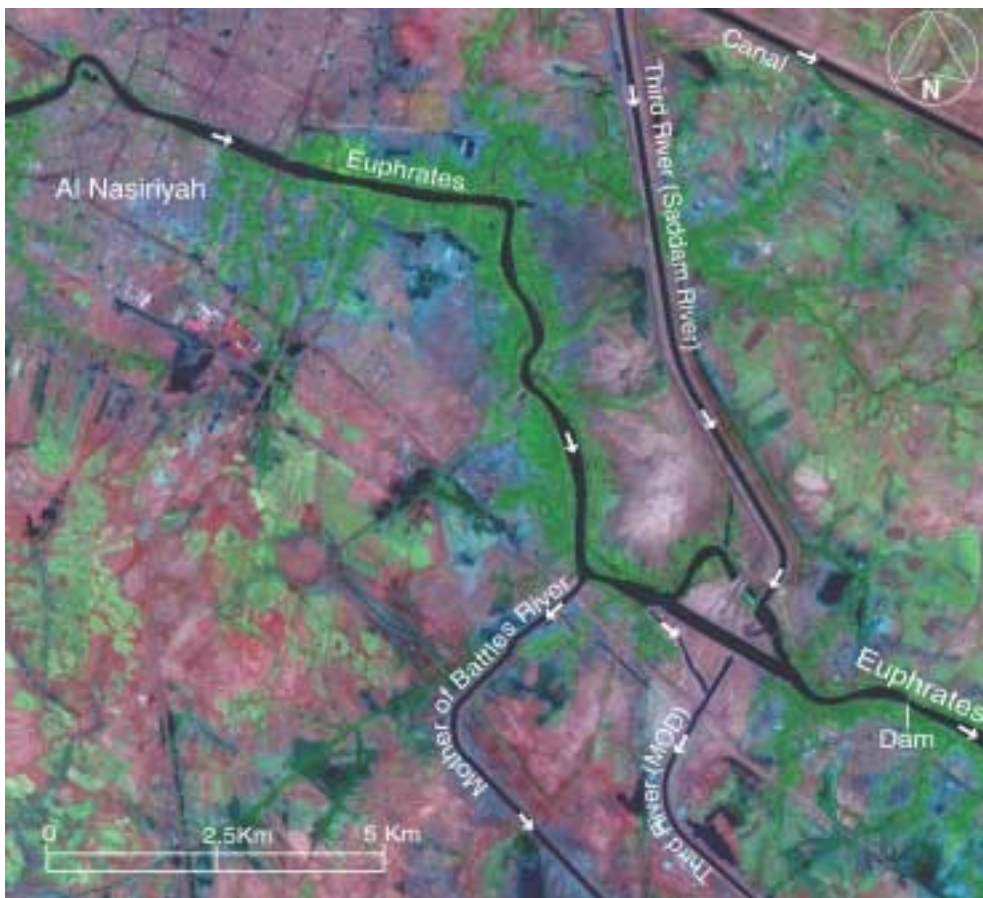
Fig. 16 - Diversion of Euphrates waters downstream of Al Nasiriyah by the twin canals of the 'Third River' and 'Mother of Battles River'. (Landsat 7 true colour image derived by merging of panchromatic ETM Band 8 with Bands 7, 4 and 2, taken on 4 May 2000).
