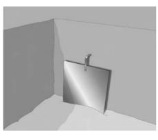
Solid copper earth plates offer a simple alternative style of earth electrode where high resistivity soil or rock conditions prohibit the driving of earth rods
