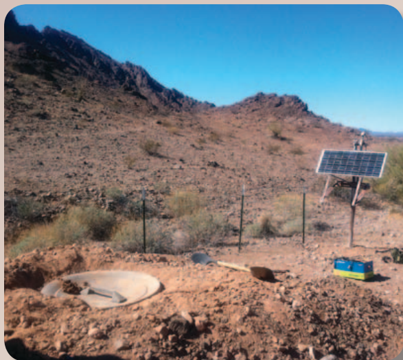
Figure 16b. Broadband seismic station of the ABSN near Yuma, Arizona.
