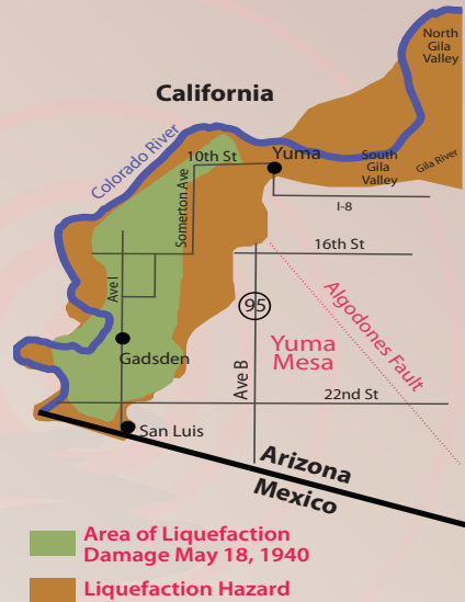
Figure 15. Liquefaction hazard zone in and around Yuma, Arizona (courtesy of the U.S. Geological Survey).
