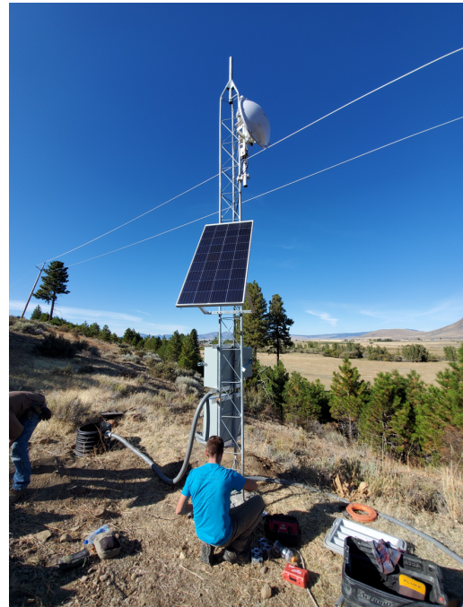
Figure 1. (left) Sugar Bowl (SUGR) EEW vault with Episensor strong motion sensor and L-4 vertical short-period seismometer. (right) Example of a typical NSL EEW seismic installation (LOYB) with solar power and microwave telemetry infrastructure.
