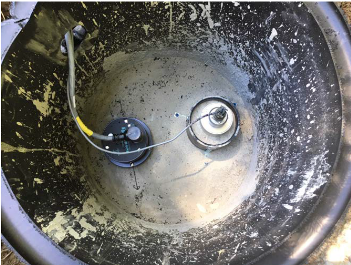
Figure 1. (left) Sugar Bowl (SUGR) EEW vault with Episensor strong motion sensor and L-4 vertical short-period seismometer. (right) Example of a typical NSL EEW seismic installation (LOYB) with solar power and microwave telemetry infrastructure.
