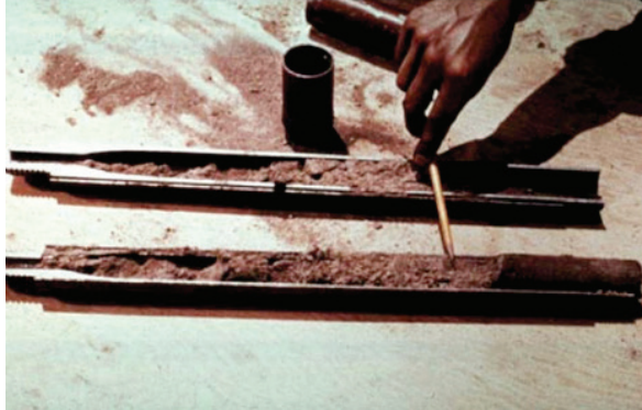
Figure 3.7: Split Barrel Sampler (Mayne et al. 2001)
