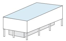
Figure 34 Out-of-plane offset irregularity.
