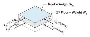
Figure 37 Required seismic design forces for Seismic Design Category A structures.
