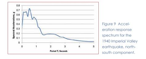
several seconds while short buildings have natural periods of a few tenths of a second. Structural engineers use the symbol T to denote the period of a structure.
