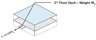
Figure 38 Continuity forces for Seismic Design Category A structures.
