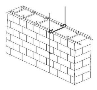
Fig 6: Containment reinforcement scheme integrated with horizontal bed reinforcement
