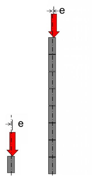
Fig. 5: (a) Short and eccentrically loaded wall (capacity < 100%) (b) Slender and eccentrically loaded wall (capacity << 100%)
