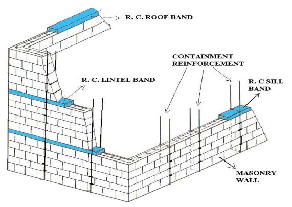
Fig 7: Schematic diagram of vertical and horizontal reinforcement in a masonry building Specification for vertical 'containment reinforcement'
