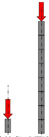
Fig. 4: (a) Short and axially loaded wall (capacity 100%) (b) Slender and axially loaded wall (capacity < 100%)
