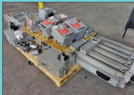
Busway and Busway Disconnects
