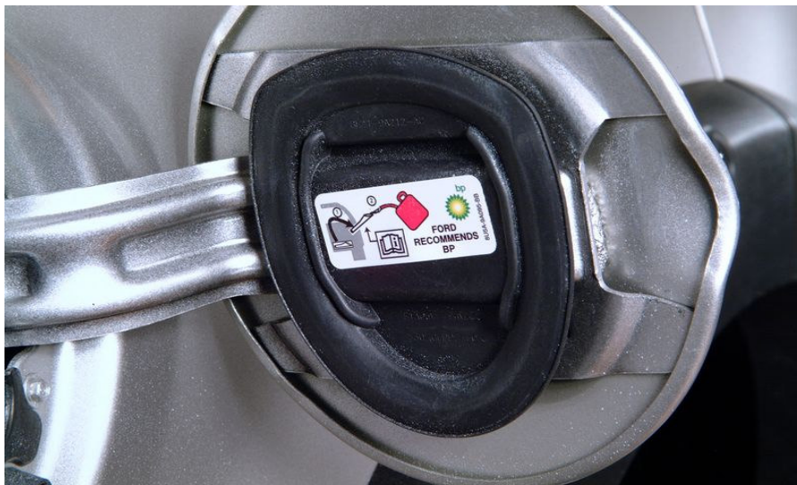
Figure 6. Outer Fuel Filler Door Seal
