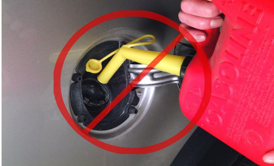
Figure 7. Do Not Attempt Adding Fuel Without the Provided Funnel
