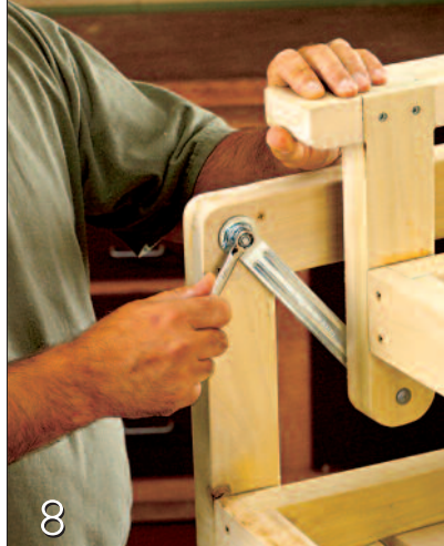
8 Fasten the swing arms with 1/4 x 2-in. galvanized or stainless steel carriage bolts and locknuts.
