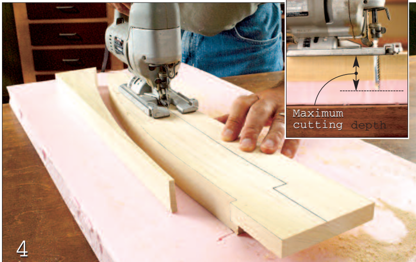
4 Cut the profiles with a jigsaw. Support the workpiece with 1-1/2-in.-thick rigid-foam insulation. The foam and workpiece must be thicker than the maximum cutting depth of the blade (see inset).
