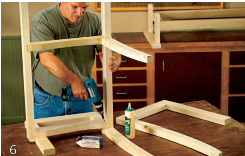
6 Assemble the base and seat frames. Fasten the joints with exterior-rated glue and screws.
