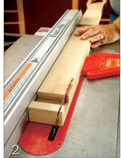
Rip a 10-degree bevel along the top edge of the front seat rail J (pictured) and the back edge of the front seat slat P, and rip a 22-degree bevel along the front edge of the top crosspiece N.
