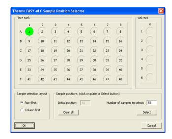
**Note** The position codes for the six extra vials on the side (Autosampler ASC) are 1-V1 to 1-V6.
