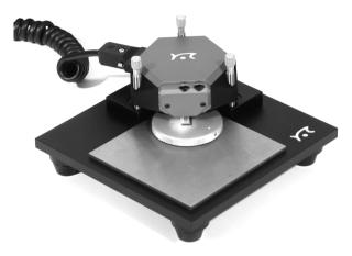
easyScan 2 AFM Scan head on the Sample Stage
