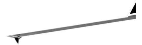
Cantilever: 228 µm long micro-fabricated silicon cantilever with integrated tip
