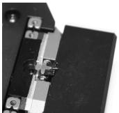
Mounting the cantilever: top left: Inserting the cantilever insertion tool; top right: Inserting/ Removing the cantilever; bottom right: Correctly inserted cantilever
