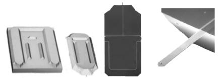
Cantilever: left: alignment system, centre: Cantilever chip viewed from the top, right cantilever 450 µm long, 50 µm wide with integrated tip.
